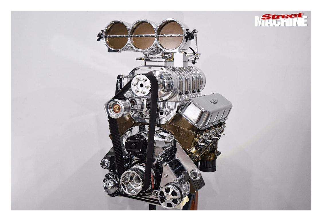
And given that the '49 is a street car – yep, a street car – the ProFlo team knocked up an in-house EFI system loaded with eight 2000cc injectors that works with the hat, so the big-block will have impeccable street manners as well as the ability to run on both E85 and pump fuel, as dictated by the flex-fuel sensor and Haltech Elite 2500 ECU. The Haltech will also manage the ignition side of the equation via an MSD crank trigger and an array of individual LS coil packs.
