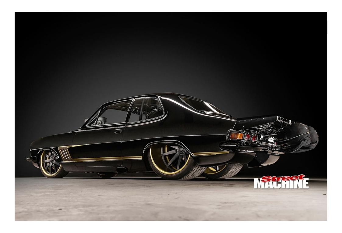
While it currently rolls on 20x7 and 24x15in Schott F10 wheels, once the LJ goes to the track it will wear 17x4.5in front-runners and double-beadlocked 15x14in hoops wrapped in 33x15in slicks out back
