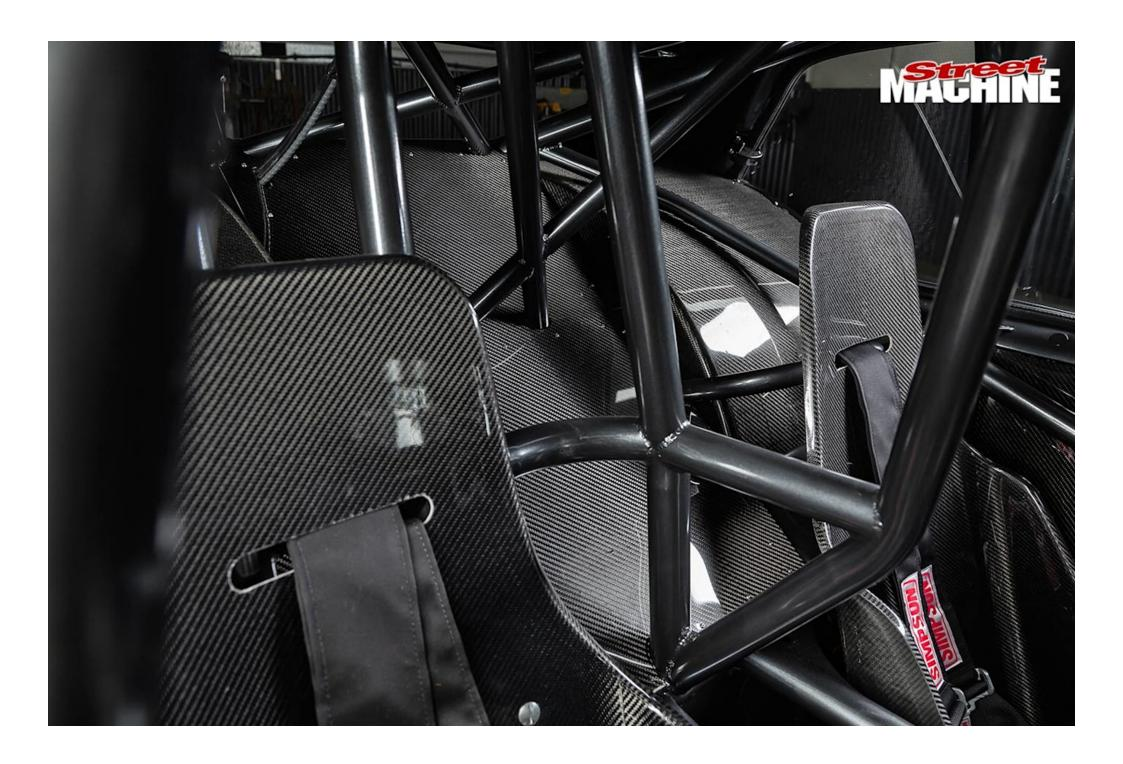
"The carbon tubs and flat sheet are JBRC race products from the USA, while the carbon seats and dash were custom-made locally," Paul says. "It is all proper carbon, which cuts weight out, and it looks sick"
