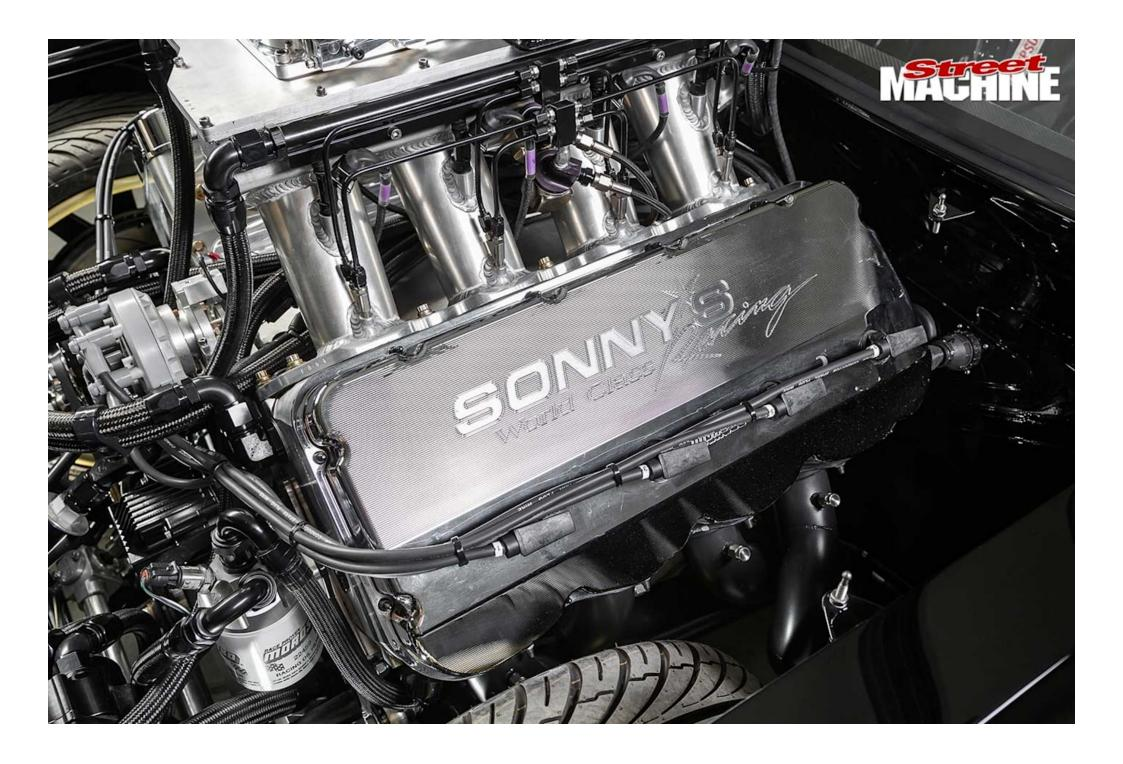
If you want to understand just how ludicrously massive this donk is, compare it to a couple of Chev crate motors. The base 350 SBC has a 4.0in x 3.48in bore and stroke, while Chev's baddest big-block, the 572ci ZZ572, runs a 4.560in bore and 4.375in stroke. The SAR940 rocks a 5.045in bore and 5.8750in stroke!
